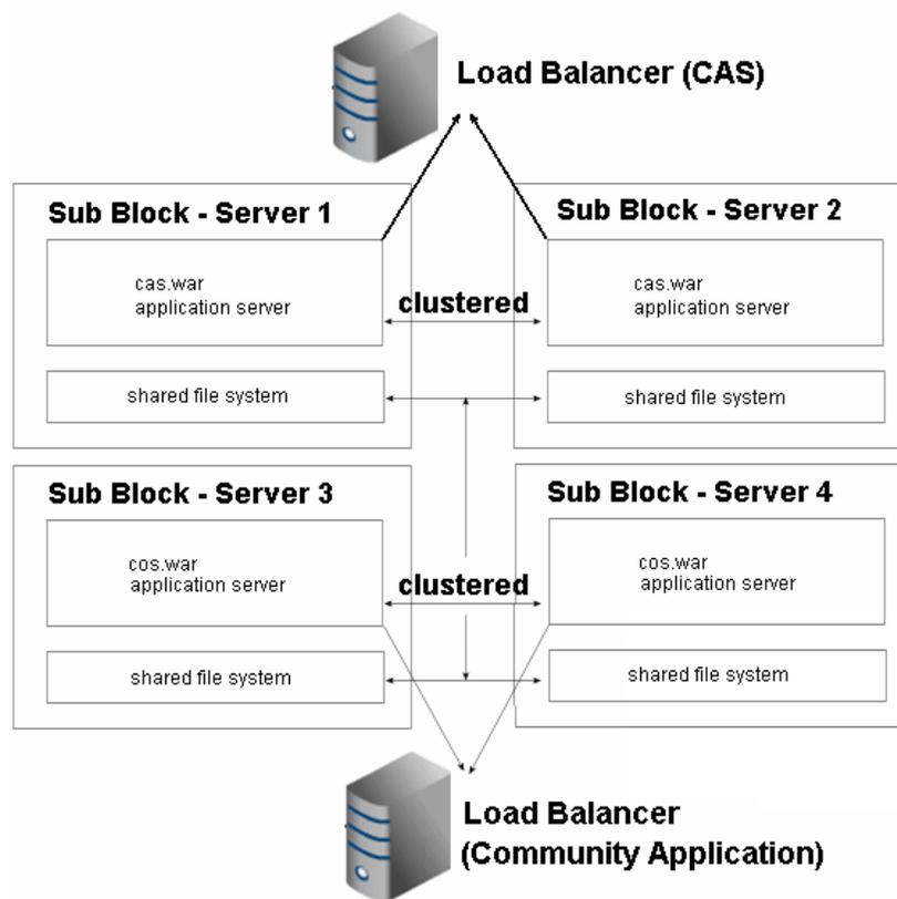
In [Figure 7](#), the Community production block (Block A in [Figure 3](#)) is divided into four sub-blocks, on four servers. The Community production block consists of two independent clusters: one for `cas.war` and one for `cos.war`. While this kind of breakdown is possible, it is not recommended. Typically, a cluster of two sub-blocks, as shown in [Figure 6](#), provides the required capabilities and failover, and with less administrative overhead.
