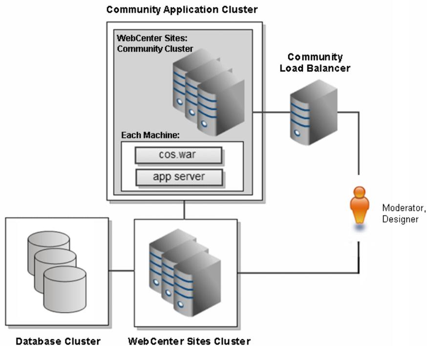
Figure 4 shows a clustered version of the management stack illustrated in Figure 3, on page 11. In Figure 4, the Community application (Block B) is now clustered. The WebCenter Sites application (Block D) is also clustered and uses a database cluster.
