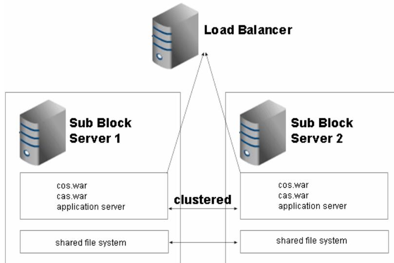
In [Figure 6](#), the Community production block (Block A in [Figure 3](#)) is divided into a cluster of two servers (which can be expanded to any number of servers simply by duplicating the sub-block, as shown in [Figure 7](#), on page 16).
