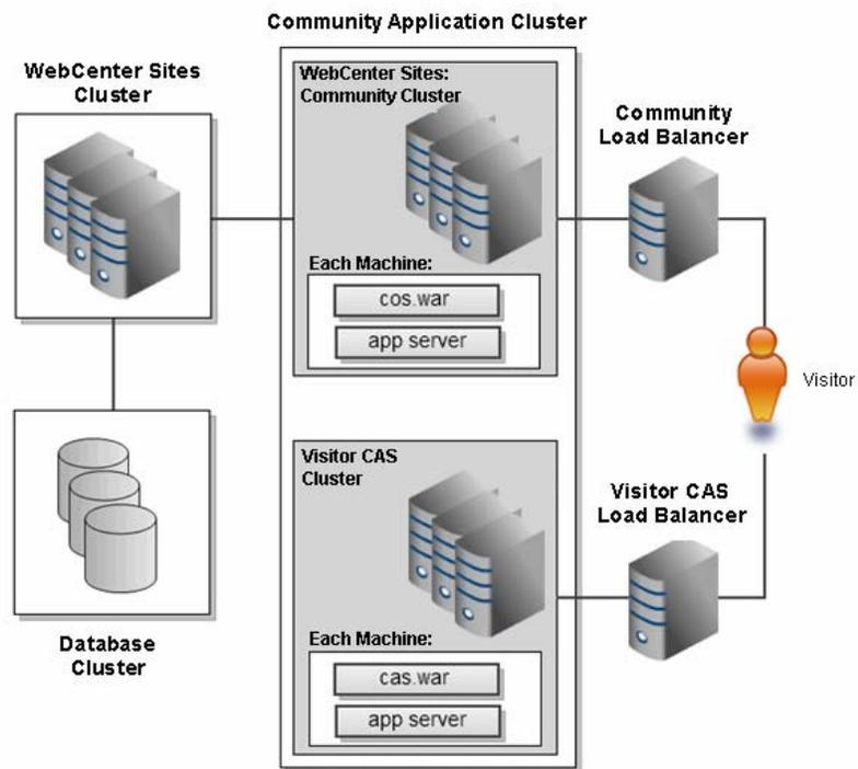
Figure 5 shows a clustered version of the production stack illustrated in Figure 3, on page 11. In Figure 5, the Community application (Block A) is now clustered. The WebCenter Sites application (Block C) is also clustered and uses a database cluster.
