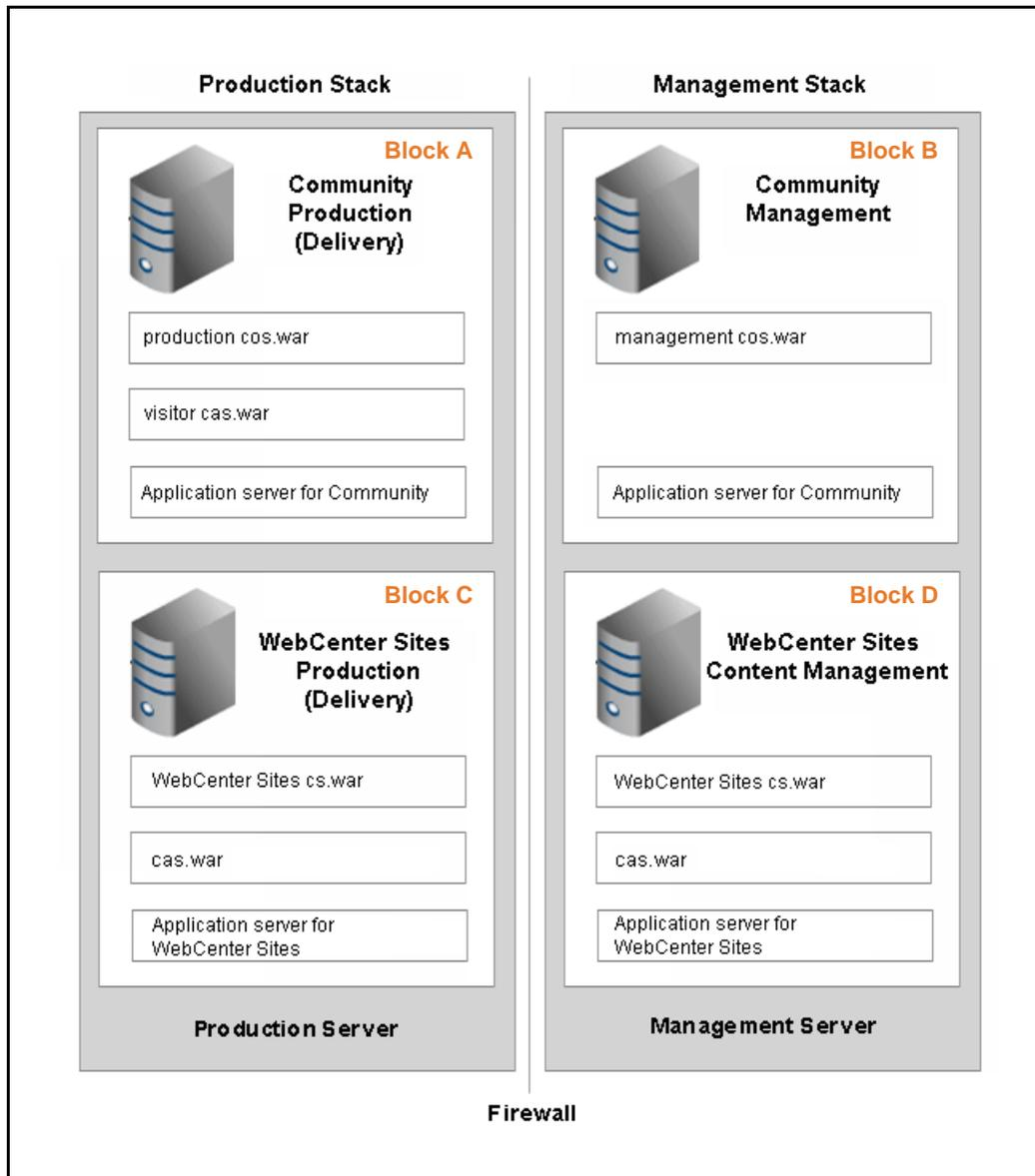
The blocks shown in [Figure 3](#) can be deployed in a number of ways, in any configuration, as long as independent application servers are used for each application inside each block.
